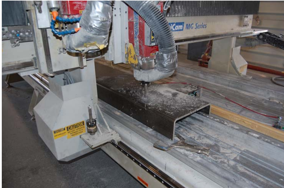
Picture 5. Factory Drilling of Holes for Hardware Connections for 287 kV H-frame Cross Arm
